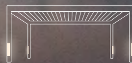
Coloured LED strips on the outside of the post at the bottom (length: 400 mm)
