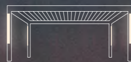
Coloured LED strips on the outside of the post at the top (length: 1,600 mm)
