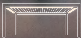
Revolving coloured LED strips at the bottom of the fascia
